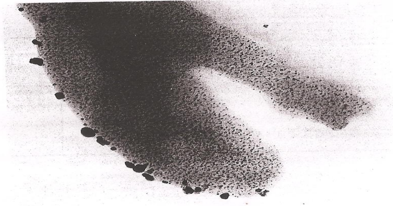
FIG. 7.17 Electron microscope photograph of platinum deposits on zeolite (1 mm = 3.3 nm).
