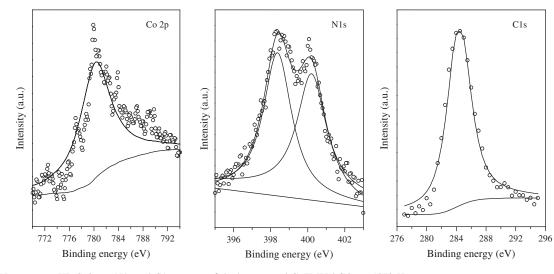
Fig. 4. Narrow scan XP  $Co2p_{3/2}$ , N1s and C1s spectra of the heat-treated CoTMPP/rGO<sub>x</sub> at 1073 K.
