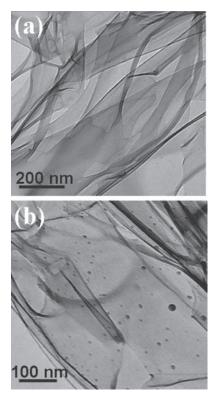
**Fig. 3.** TEM images of (a)  $rGO_x$  and (b) heat-treated CoTMPP/rGO<sub>x</sub> at 1073 K.
