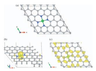
**Fig. 6.** (a) DFT optimized structure of  $\text{CoN}_4$  doped graphene substrate and the frontier ((b) valence (c) conductance) bands. The isosurface value used is 0.001 e/Å<sup>3</sup> (Color code: Green corresponds to cobalt, blue to nitrogen and grey for carbon throughout this manuscript).
