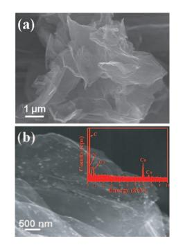
**Fig. 2.** SEM images of (a)  $rGO_x$  and (b) heat-treated CoTMPP/rGO<sub>x</sub> at 1073 K. Inset in Figure 1(b) shows the corresponding EDX spectrum.
