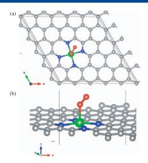
**Fig. 7.** Top and side views of most stable configuration of  $O_2$  on  $CoN_4$  doped graphene.  $O_2$  prefers bonding to on-top of Co atom. (red balls correspond to oxygen).
