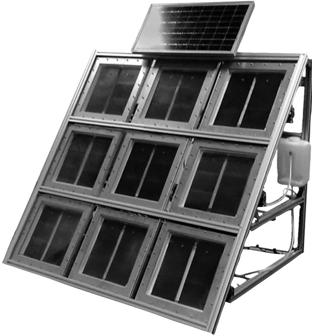
Fig. 8.1 Demonstration model of a 1-m 2 PEC array
