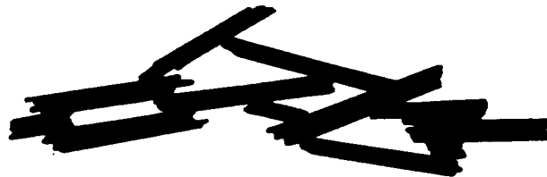
Fig. 1.9 Pores in an aggregate composed of plate-like particles.
