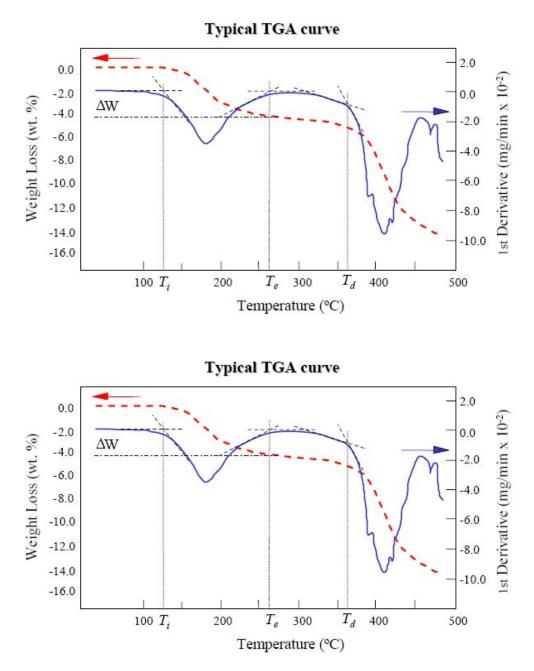
Fig. II.1 Typical TG curve shown in red (dotted line) and DTG representation given by the continuous line in the figure.
