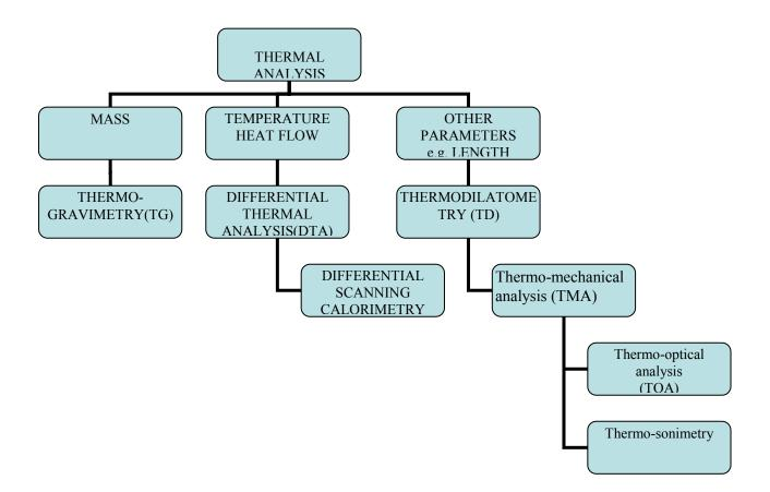
Fig.1.1. Thermal Analysis refers to a number of methods that measure change in any property of a system with respect to temperature, when it is subjected to a controlled temperature variation. The measured parameters can be mass, temperature or heat flow or other properties, dimensions, or optical or magnetic property.
