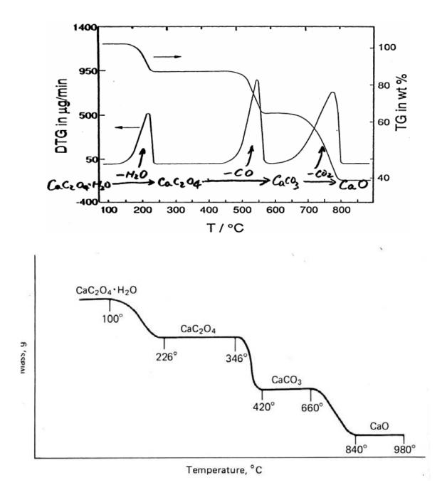
Fig.II.2. Thermo gravimetric trace for the decomposition of calcium oxalate (one can notice that the trace provides information on the steps and also the species involved in the decomposition process).
