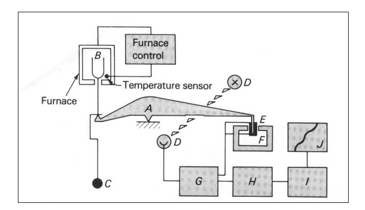
Fig.2.1. A schematic diagram of a typical thermo gravimetric apparatus [ A – beam; B – Sample cup; C –Counter weight; D – Lamp and photodiode ; E – Coil; F – Magnet; G – control amplifier; H – Tare calculator; I – Amplifier J – Data station]
