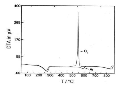
DTA curves for the thermal decomposition of  $\text{CaC}_2\text{O}_4\cdot\text{H}_2\text{O}$  at 20 °C min^1 in  $\text{O}_2$  and Ar
