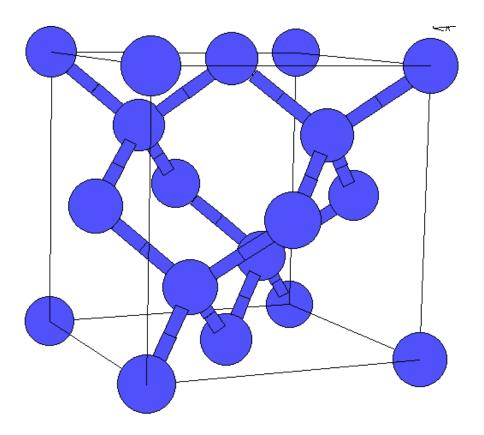
In Si crystal, each atom is connected to the four neighboring atoms by covalent bonds.
