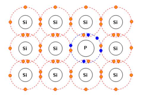
A silicon lattice with a single impurity atom (Phosphorus, P) added.
