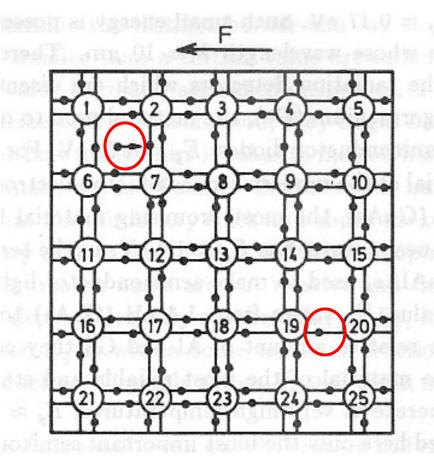
When the electron leaves the Si atom, it is lacking one electron.
