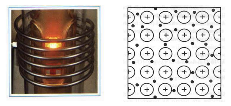
In metals, the atom-to-atom interactions free up one electron from each atom. The metal crystals have as many free electrons as they do atoms.
