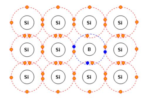
A silicon lattice with a single impurity atom (Boron, B) added. Boron has only three valence electrons, one electron less than the Si atom. Having only three valence electrons - not enough to fill all four bonds - it creates an **excess hole** that can be used in conduction.
