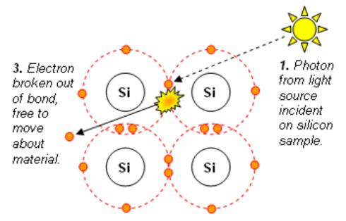
**2.** Photon collides with electron in a bond (Valence Band). The Photon's energy is given to the electron, pushing it up into the Conduction Band.
