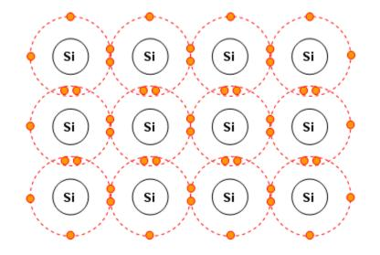
Si crystal lattice structure, showing the valence electrons associated with each bond.
