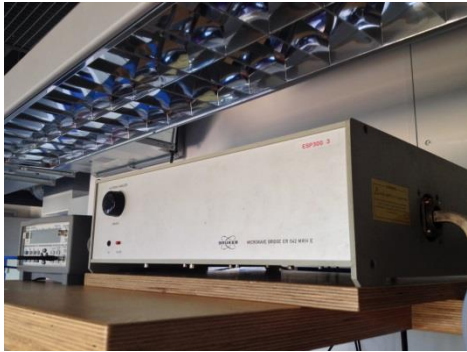
Microwave Source System
