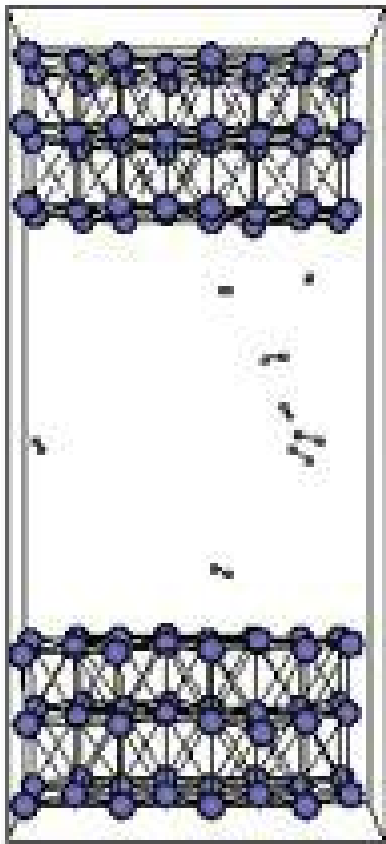
8 H 2 -molecules in contact with a perfect 96-atom (111) Pt-surface. MD-simulation at 298K
