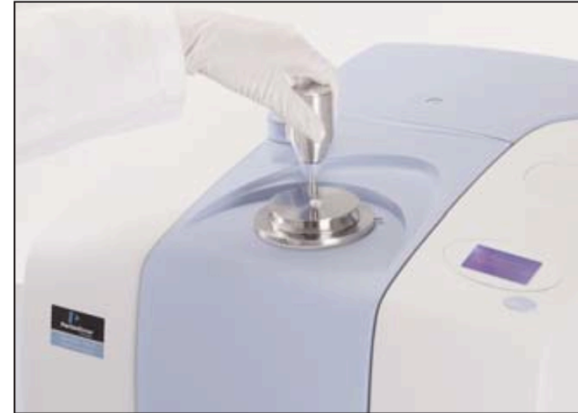
Figure 7. Applying pressure to a solid sample on the Universal diamond ATR top-plate.
