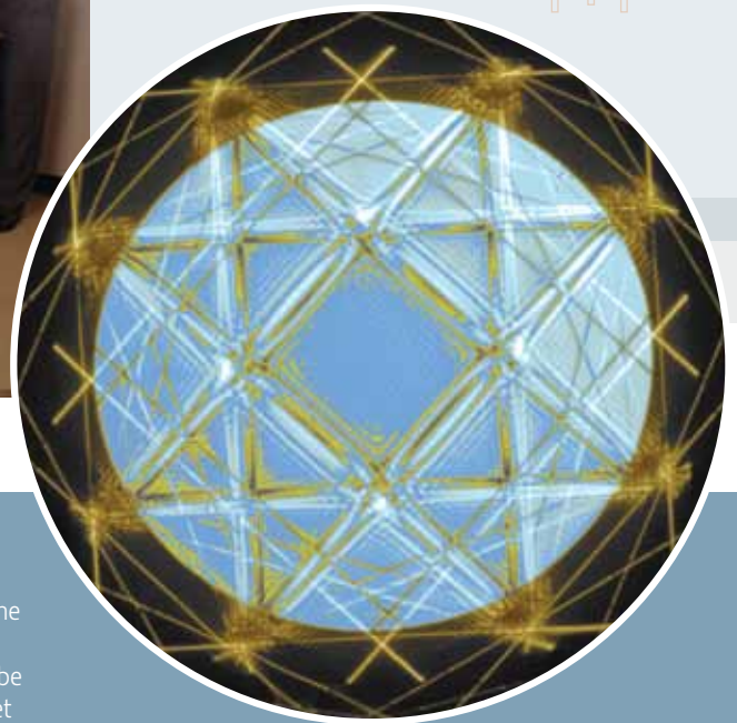
Large Angle Convergent Beam Electron Diffraction (LACBED) pattern from a diamond.
