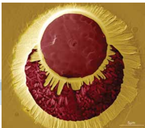
FIB-cut in steel v2a EE by 1nA to IB milling-002 steel.
