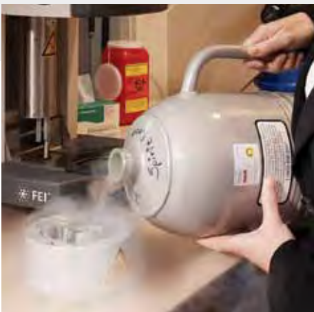
Applications specialist preparing the coolant container with liquid nitrogen and loading a sample onto the grid.
