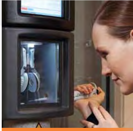
Applications specialist preparing the coolant container with liquid nitrogen and loading a sample onto the grid.
