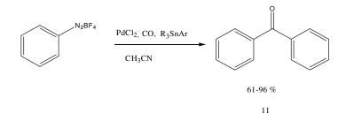
The other product of the reaction was probably F-SnR<sub>3</sub>. In the synthesis of diaryl ketones 11 the reaction was very selective: no products containing any alkyl group from Ar'SnR<sub>3</sub> were observed. Furthermore, neither symmetrical ketones (ArCOAr or Ar'COAr') nor biaryls were formed.
