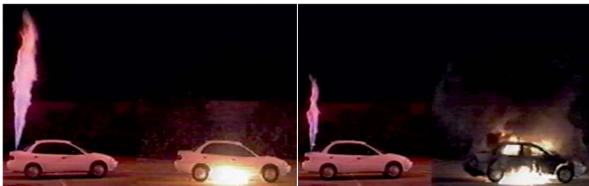
Figure 1–2. Hydrogen jet fire and gasoline fire: 3 (left) and 60 (right) seconds after car fire initiation (Swain, 2001).
