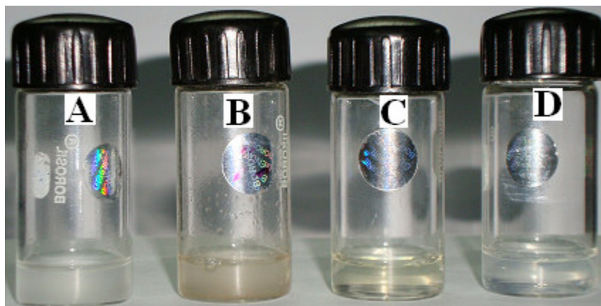
Figure 5.4. Color of the samples [A-pure core (sulfur), B-core-shell (S@AgBr), C-mixture of pure sulfur and AgBr and D-pure AgBr particle] for 5 mM thiosulphate and 0.1 mM AgNO 3 concentrated solution.
