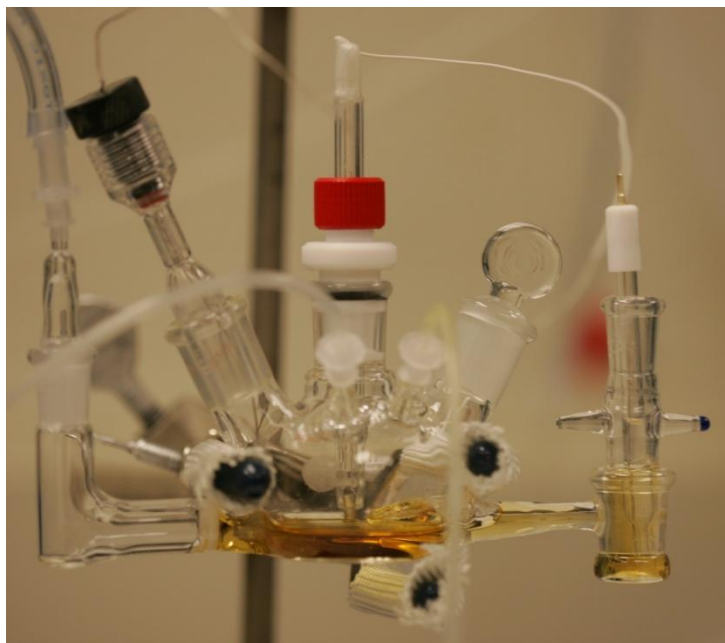
Figure 3.2: Picture of Electrochemical Cell filled with 1-Ethyl-3-Methylimidazolium Tetrafluoroborate (EMIM BF 4 ) with a Gold Working Electrode.
