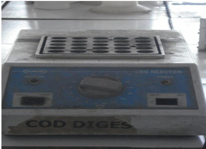
Fig-3.4 COD digester
