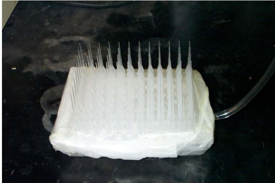
**Figure 1.2c** Homemade Multipipette delivering solutions of 0-20  $\mu$ l
