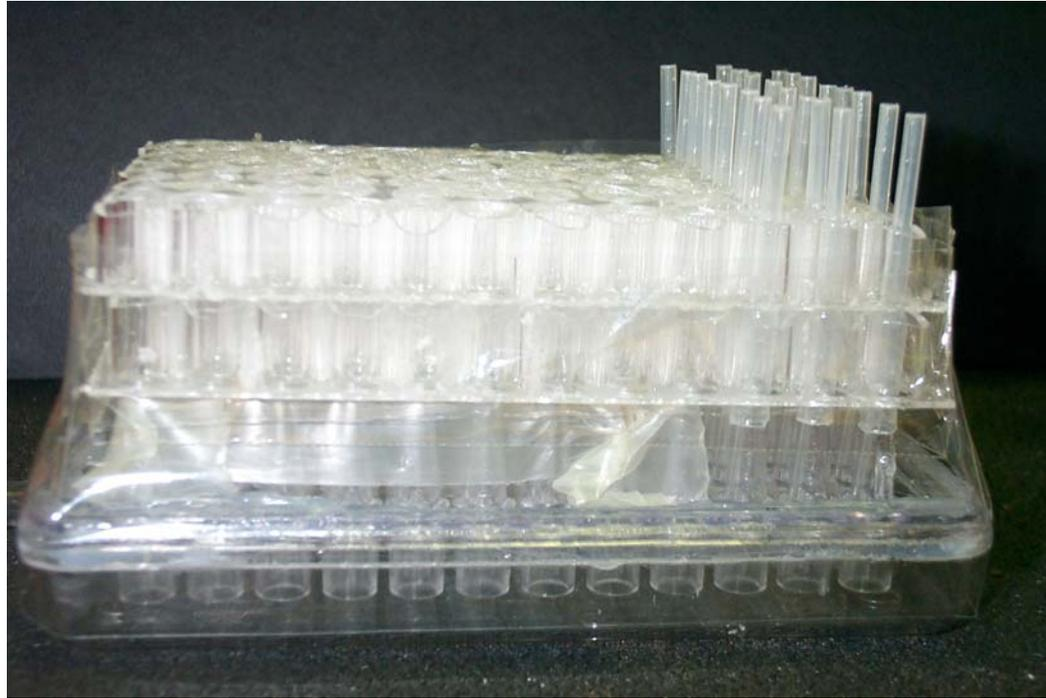
**Figure 1.2b** A modified home made device for sorting beads along rows
