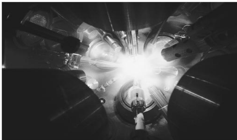
Fig. 4.1. Lasers focus on a small pellet of fuel in attempt to create a nuclear fusion reaction (the combination of two nuclei to produce another nucleus) for the purpose of producing energy (reproduced from ref. 1)
