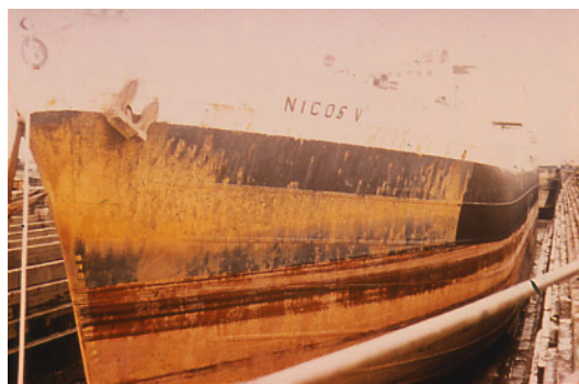
Fig . 11.14. Corrosion of ship by sea water
