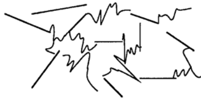
Fig. 2. Sketch of the “Open Structure” with Extensive cross linking and small aromatic ring systems (reproduced from ref. 4)
