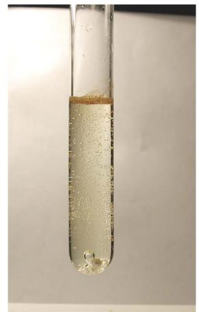
H<sub>2</sub> gas bubble evolution from the heavy metal halide reaction.
