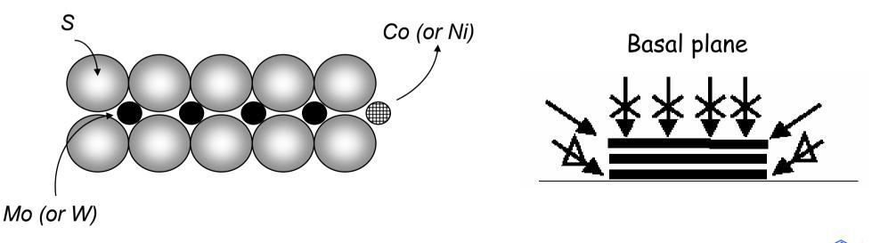
The steps of the guided formation (molecular design) of the nanocomposite, completely sulfided bimetallic active phase (BIC apprach)
