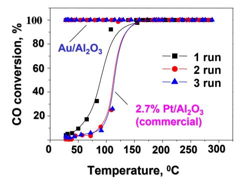
Flow reactor;  $0.1\%CO + 14\%O_2 + 10\%$  of H<sub>2</sub>O (N<sub>2</sub> for balance); Heating rate of 10 K/min; SV = 50 l/h
