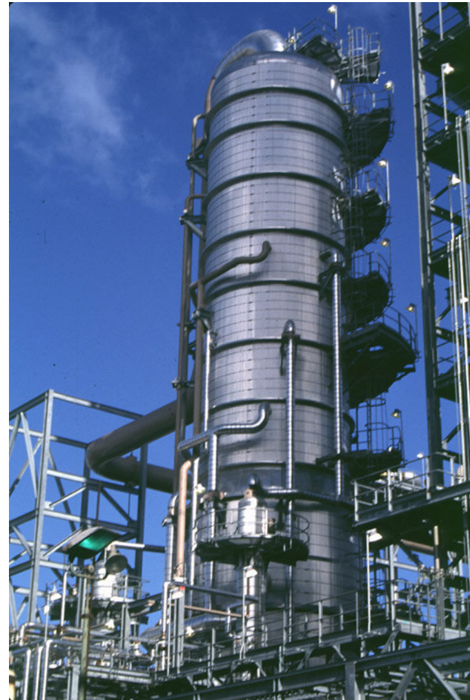
Industrial scale fluidized bed catalytic cracker for gasoline production
