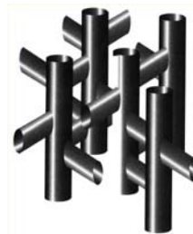
17.12 The structure of ZSM-5 has intersecting channels defined by the crystal structure. The tubes in this diagram represent the channels with the three-dimensional structure.
