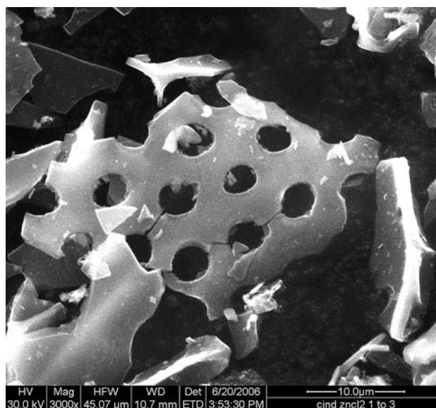
Fig. 12 SEM image of activated carbon from Calotropis gigantea activated with \text{ZnCl}_2 (wt/wt% ratio of Char: \text{ZnCl}_2 is 1:3; from ref. [25])
