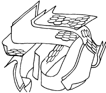
Fig.1. Structure of Activated Carbon - A schematic representation (reproduced from ref. 6)
