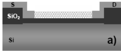
Fig. 6. Schematic side view of a back-gated SWNT-FET with 10 nm thick SiO 2 gate dielectric under the channel and 100 nm SiO 2 under the bonding pads
