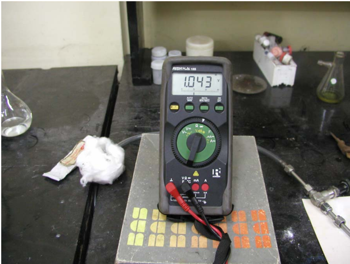
Fig.7. The measurement of voltage developed by the Fuel cell.
