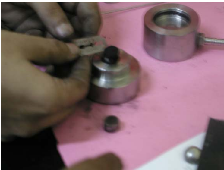
Fig.3 & 4 : Pellet press used for preparing the electrode.
