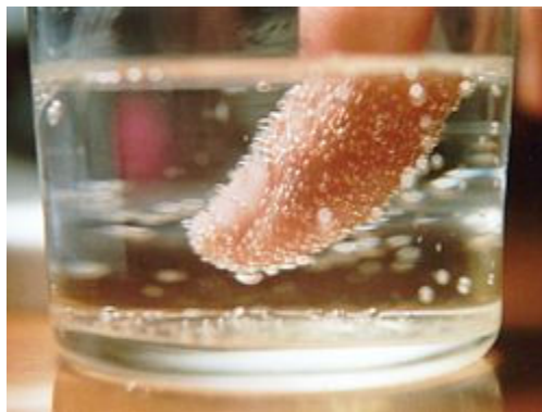
Fig. 4.3. Nucleation of carbon dioxide bubbles around a finger (ref. 5)
