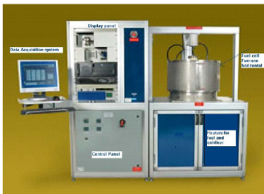
Control Panel for the fuel cell
