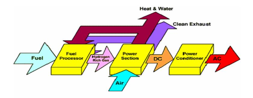
In addition to the above, a number of other sub-systems (viz.: Fuel storage & delivery system, Air supply system, Thermal Management system, C&I systems etc) are also needed
