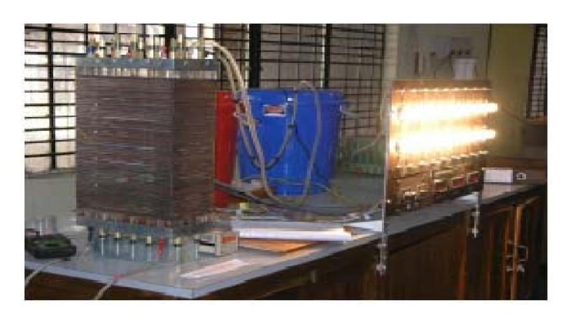
50 Cells, 150x300 mm, PEMFC 1 kW modular stacks
