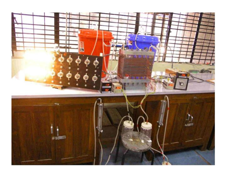
50 Cells, 150x300 mm, PEMFC 1 kW modular stack (under testing - January 2006)
