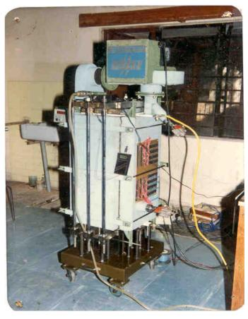
(5 kW PAFC stack under testing, Active Area 865 cm<sup>2</sup>, 1995)
