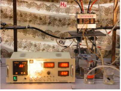
(PEMFC, 20 cells' stack under testing - Nov 2005)
