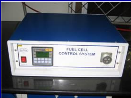
Fuel cell Control system
