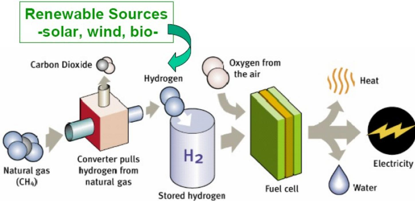
The ultimate potential is generation of off-grid electricity from hydrogen produced from completely renewable, widely dispersed energy sources.
