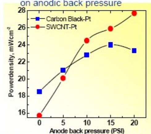
MEA was prepared by electrophoretic deposition of Pt black on varying amount of SWCNTs
