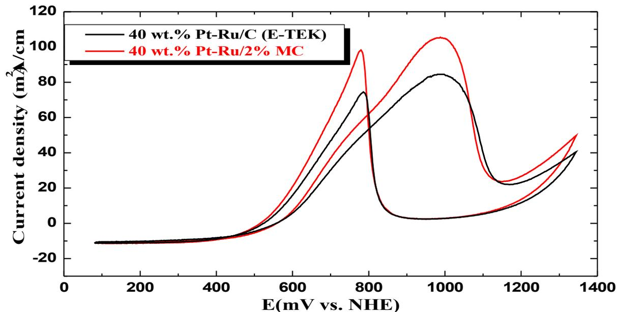
Cyclic voltammograms of prepared catalysts for the electrooxidation of methanol in 0.5M H<sub>2</sub>SO<sub>4</sub> + 1M CH<sub>3</sub>OH with a scan rate of 25mV/s & scan cycle of 30.
