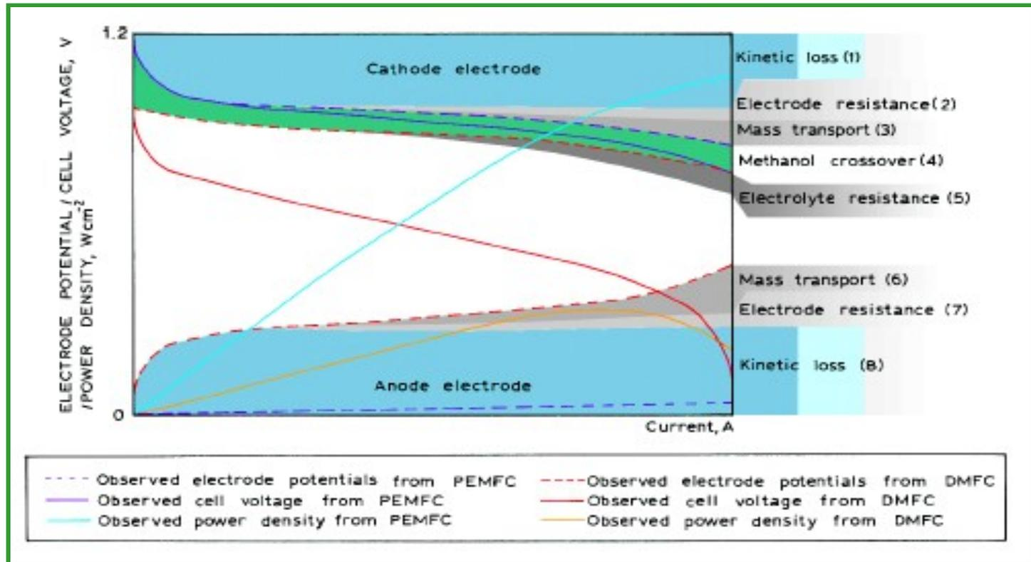
Performance losses seen in a typical DMFC MEA operating with dilute MeOH & Air at 80°C, compared to those in a PEMFC
