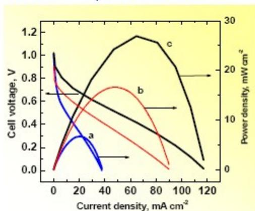
Dependence of power output on anodic back pressure
